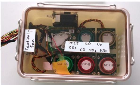
Fig.5 An instrument for the measurement of PM<sub>2.5</sub> and trace gases (CO, CO<sub>2</sub>, NO., NO<sub>2</sub>, and SO<sub>2</sub>)
