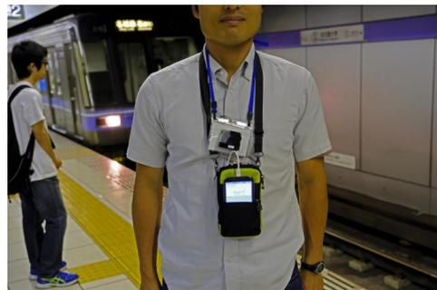
Fig.1. Snapshot at a subway station during a one-day personal exposure measurement using our PM<sub>2.5</sub> instrument.
